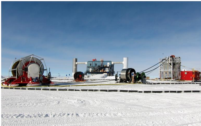
The IceCube hot-water drilling rig set up at South Pole Station. Credit: Jim Haugen, University of Wisconsin.
