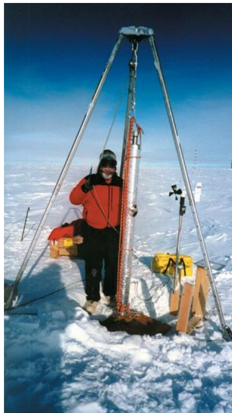
Global Seismic Station SPA at South Pole, Antarctica. Shown is a prototype borehole sensor package being tested in a shallow vault. This prototype was eventually deployed at the new South Pole seismic station QSPA, located 5 miles from SPA. Credit: IRIS
