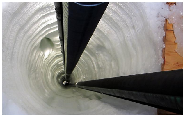
View down one of IceCube's deep ice holes during hot-water drilling. Credit: Jim Haugen, University of Wisconsin.
