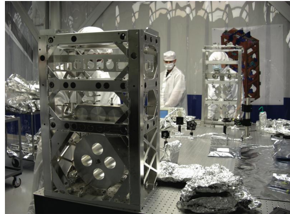
Assembly and testing of AdvLIGO optical suspension components for use in high vacuum. Credit: LIGO Laboratory.
