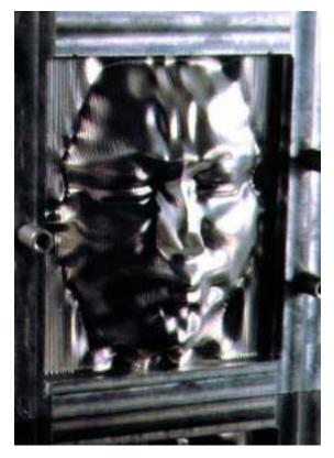
NSF-funded researchers at the University of California at Berkeley, have created an experimental system called CyberCut that allows users to quickly design and manufacture prototypes for mechanical parts via the Internet. An online computer modeling tool links to a computercontrolled milling machine. Here, Cybercut renders art—a human face scanned by lasers.
