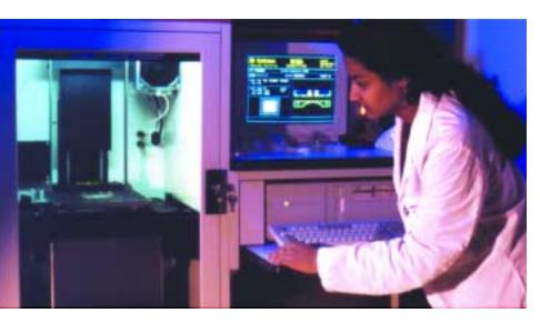
NSF helped launch rapid prototyping technologies, which can build new products from a computer-aided design (CAD) model without any carving or machining. Here, a student works with rapid prototyping equipment in the NSF-supported Advanced Design and Manufacturing Laboratory at the University of Maryland. One goal of the lab is to create graphical materials for visually impaired students.
