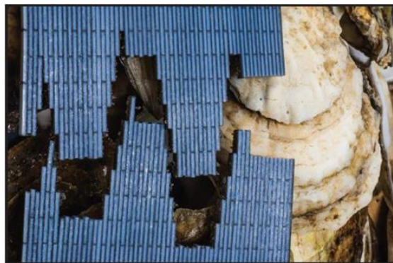
Figure 2. Bioinspired artificial mesoscale materials created by 3D ink-jet printing of two polymers, one soft and one stiff, based on the brick and mortar structure of nacre and bone. One of these materials demonstrates fracture resistance up to 22 times that of its strongest constituent.
