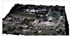
The earthquake that struck Haiti in 2010 destroyed the National Palace in Port-au-Prince. This image combines high-resolution imagery and structural measurements, and uses laser pulses to make 3-dimensional elevation measurements. Credit: Rochester Institute of Technology
