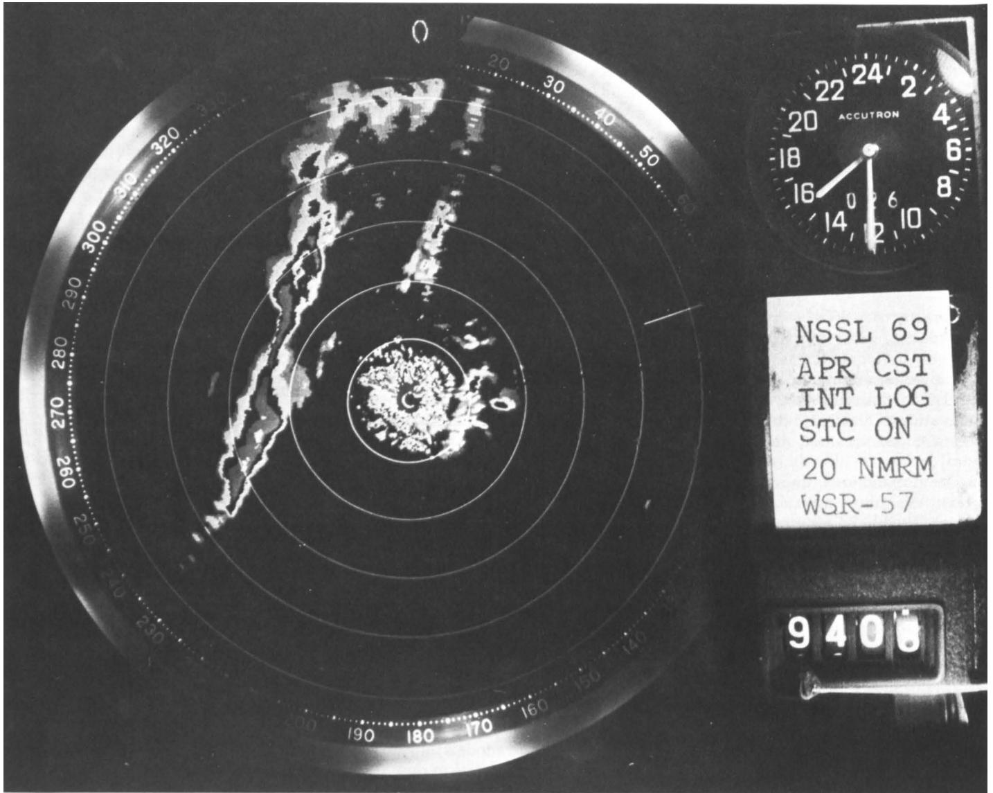
The figure shows the PPI-scope of the 10-centimeter WSR-57 radar at the National Severe Storms Laboratory in Norman, Oklahoma on April 26, 1968. Differences in shading indicate intervals of a factor of 10 in received echo power. From such an electronic display it is possible to determine the most dense part of a storm. Range marks are at intervals of 20 nautical miles. North is at the top of the figure.
