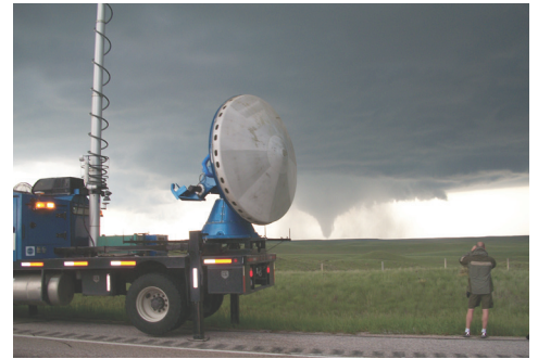
Mobile Doppler radar gathers more precise data about severe weather events in near-real-time.
