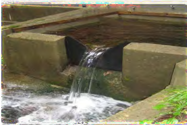
A gauging station at Hubbard Brook provides new data on acidification of streams.
