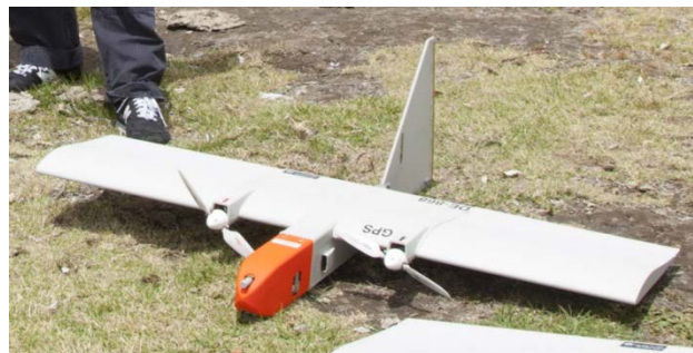
Repurposed DragonEye UAV showing the SO 2 sensor (side), barometric pressure, temperature, and humidity sensors (front) used at Turrialba, Costa Rica. Photo credit: Justin Linick, JPL
