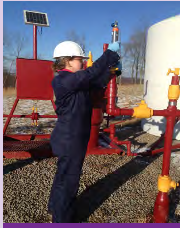
▲ Student collecting gas samples from the well-head of a producing well. CREDIT: S. SHARMA, WVU
