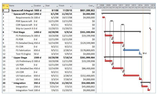
This is a project starting June 1, 2008, with a ship to launch site end date of November 20, 2015. The project cost is estimated at \$651.6 million.<sup>2</sup> Resources are shown on the bar chart and include mostly labor, with some equipment in the First Stage and Upper Stage Fabrication activities.
